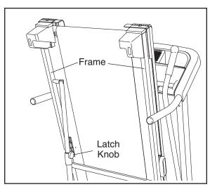
2. Hold the metal frame firmly with both hands and lower it to the floor. CAUTION: Do not grip only the plastic foot rails or drop the frame to the floor. Bend your legs and keep your back straight.
